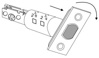
To convert the backset back to 2-3/8", simply rotate the Latch Front, Snap and rotate back till the Inner Housing Lug **"clicks"** inside the 2-3/8" Window.
